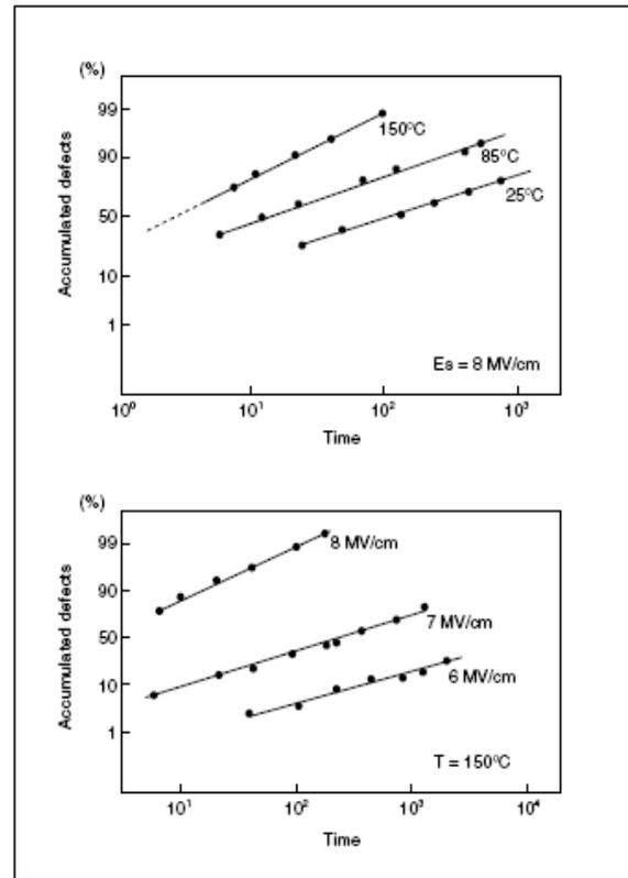
**Figure 2 Time Dependent Dielectric Breakdown**
